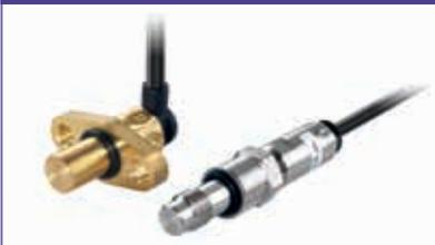
For applications that expose the sensor to particularly high pressures, RHEINTACHO developed special speed sensors with a heavy-duty design, either with brass or stainless steel housings. Sensors that have to be used in machines, such as orbital motors, must meet the highest requirements. Our high pressure sensors comply with protection classes IP69K and IP67, operate over a wide frequency range and guarantee high EMC stability.
